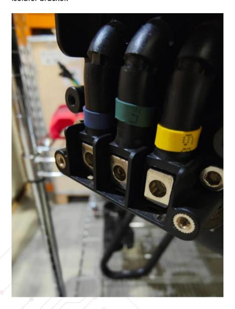
8. Finalize the installation by using a screwdriver to securely tighten the connection. The use of Loctite 243 on the screw is advised.
